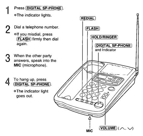
•While using the speakerphone, if the handset is on the base unit, you may switch to the handset by lifting it up.
